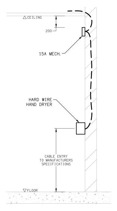
**DETAIL** HAND DRYER CONNECTION NOT TO SCALE
